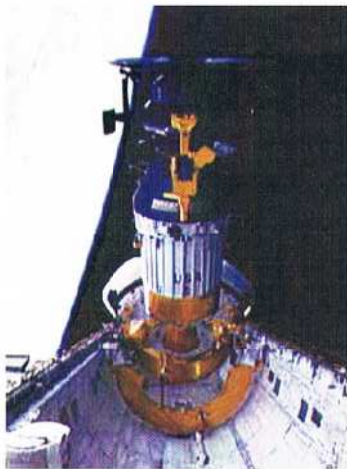
The Galileo spacecraft, carried aloft by the shuttle, weighed 2.5 tons. The shuttle can carry as much as 55,000 pounds of payload into an orbit about 100 miles high. The higher it goes, the less it can carry. At 320 miles above Earth, the shuttle's payload capacity drops to about 20,000 pounds.
