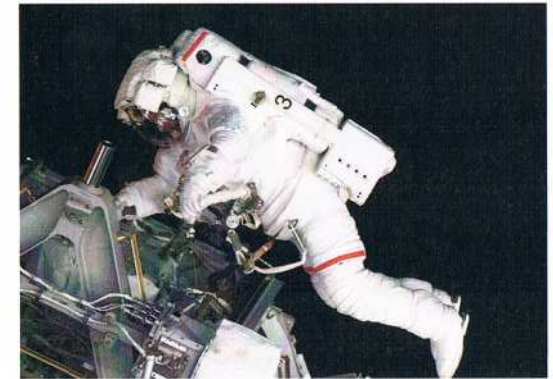
Crew members wear small gas jetpacks that can get them back to the station if they get separated from the spacecraft.
