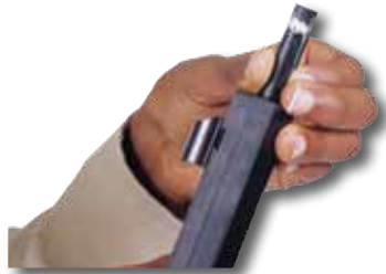
Check the bore for a load.
