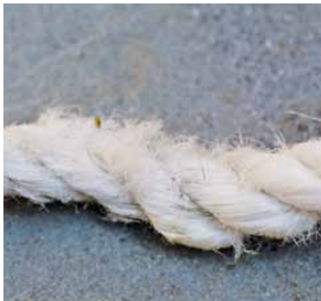
Damaged—and therefore unusable—rope
