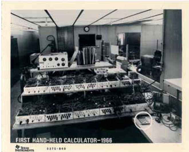
The breadboard (construction base) for the first electronic hand-held calculator fills a room.
