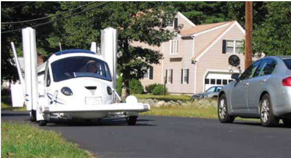
The Transition roadable aircraft is a plane that can fold its wings and be driven along the road like a car.
