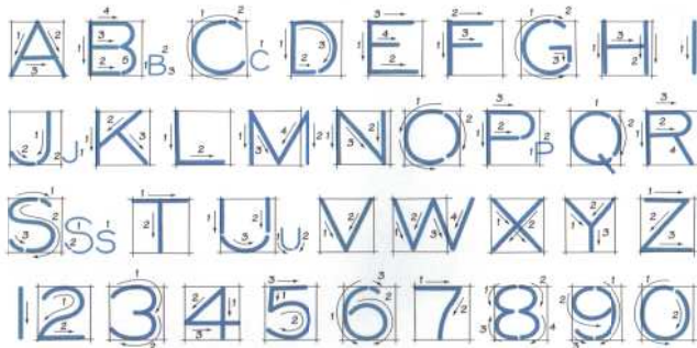
Mechanical and electrical lettering
