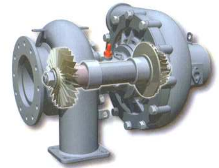
A sectional drawing or "cutaway view" shows objects inside a larger object.
