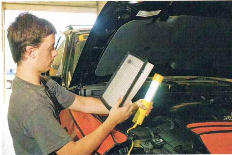
Checking the air filter
